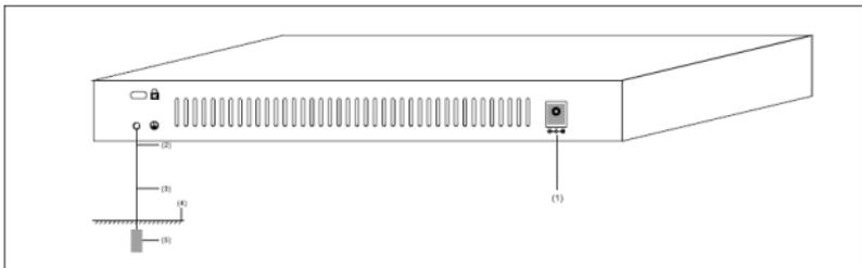
Figure 2-5 Install with a ground conductor buried
