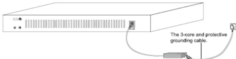
Figure 2-6 Install with the grounded power cord
